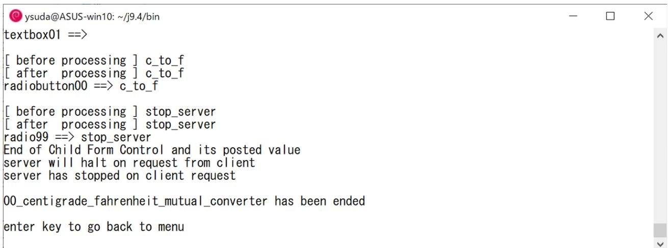
Figure 26: This is the screen shot of the server jconsole on receiving halt request. The web form application stops and the server waits for enter key to go back to main menu.
