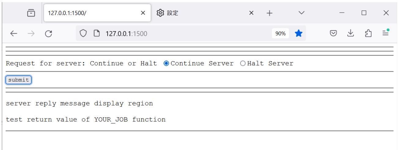
Figure 2: The screen capture of the HTML document received after submission. Note the content of the server reply message display region at the bottom of the document shows test reply message which is returned YOUR_JOB function written in the definition file.
