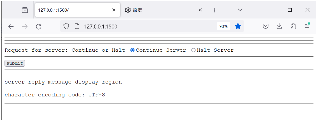
Figure 1: This is the core structure of the web form server. The radiobutton for server activity control, i.e. continue or halt and submit button are parts of the core structure of HTML document. This core document is created by the system in the process of creating web form application. There is no need of writing HTML source in the definition file for web form application.
