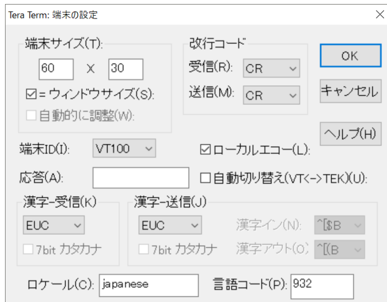
Figure 11: In teraterm, local echo option is needed because the simple server does not echo back keyin characters in real time.
